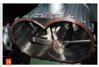
The mode of operation of the mixer/kneader affords a short time, usually less than 5 minutes, with high mixing accuracy and careful handling of the mixture.
