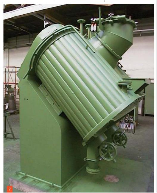
The requirements for a mixer which mixes the material as carefully as possible within short time featuring sealing problems as few as possible have been met for years by developing the Slanting Mixer Type  $\underline{VI}$  S. By arranging the mixing trough under 45 degrees it is possible to move the product horizontally, vertically and radially by means of a slow moving mixing blade. The main conveying direction is always to above into the free space, i.e. the material is very carefully moved.
