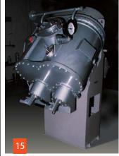
AMK Slanting Mixer/Kneader with cutting/dispersion blades are used, whenever agglomerates have to be broken down, be they nodules or of irregular dampness. In many cases the cutting blades obviate the necessity of nozzle feed or spray attachment. One or more cutting blades can be fitted per mixing arm.
