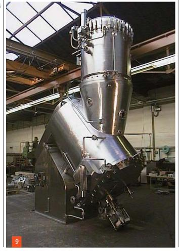
The trough, the front surfaces and the feeding opening are jacketed for heating by steam, water or heating oil. The vacuum nozzle is arranged at the highest possible part of the trough.
